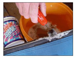
A leaking zip can hardly ever be repaired. Carefully examine the sealing surface around the inner elements on both sides for damage to the material itself or signs that the inner elements are not holding together. If you find a problem here it probably means replacing the zip so contact us and your bank manager immediately.
