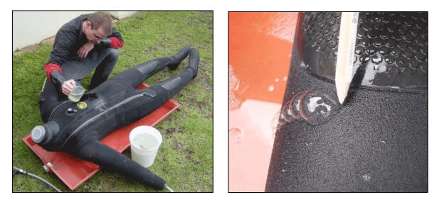
Be aware that some small leaks only allow flow in one direction (outside to inside) and when you test the suit normally you are looking for inside to outside flow. So one-way leaks will not show unless you use the same method with the whole suit inside-out.
